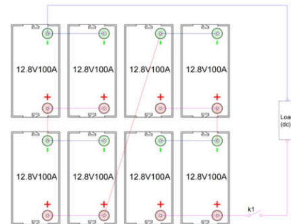
Figure 5-4 Series-parallel Applications: 4S2P,51.2V200Ah
